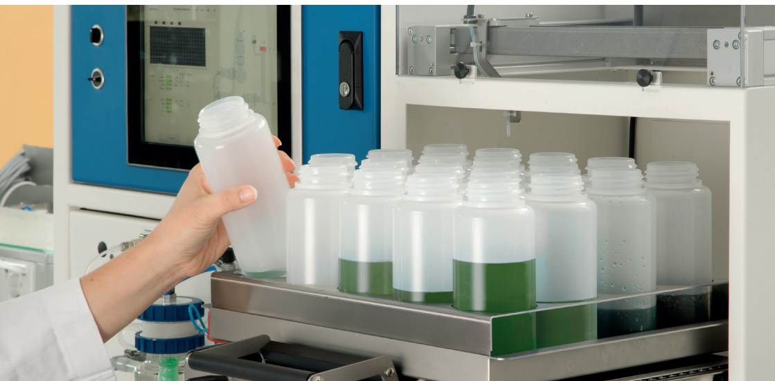
Figure 6. Sampling module (number and size of sampling bottles is flexible).
